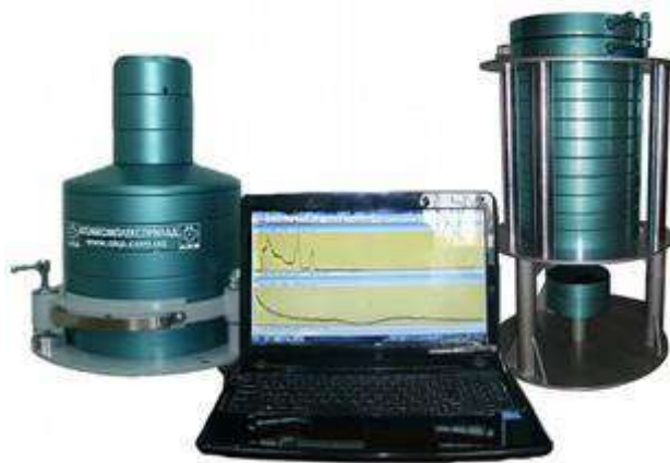
Gamma-spectrometer Seg-001 "AKP-S"-63 produced in 2017( 1dv)
