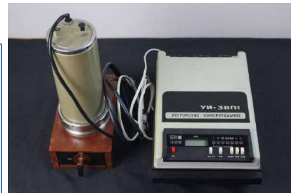
Beta- radiometer RUB-01 produced in 1991 (5 dv)
